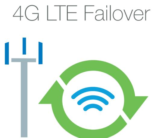
During a network interruption, a cost-effective 4G LTE backup link is automatically activated to maintain connectivity. The 4G circuit is powered by SD-WAN, so you can control what internet traffic has priority. When the primary circuit recovers, the 4G link returns to stand-by mode.
