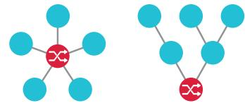
should take care to keep any Ethernet device from being more than three hops away from a network gateway.
