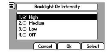
**4.** Use the △ or ⊲ to select high, medium, low, or off and press the **Select** soft key to modify the Backlight On Intensity.
